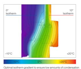
Due to the deep glass position, tremendous construction depth and the directly glued window panes glazing LIGHT ( $U_g = 0.5 \text{ W/m}^2\text{K}$ ) can achieve a sensational  $U_w$  value of 0.68 W/m<sup>2</sup>K (with ISO spacer).
