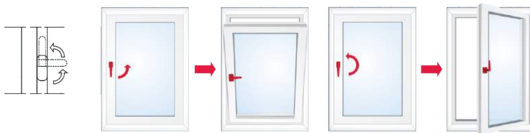
Tilt and turn window (closing - tilting - turning)
