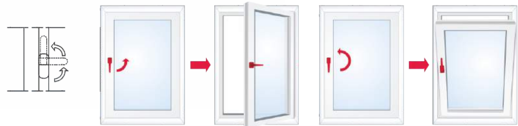
Turn and tilt window (closing - turning - tilting)
